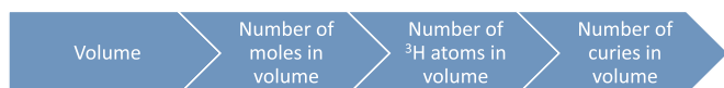
Fig. 8. Model block diagram of radioactivity (Ci) calculation for tritiated nitroxide and titanium tritide volumes.
